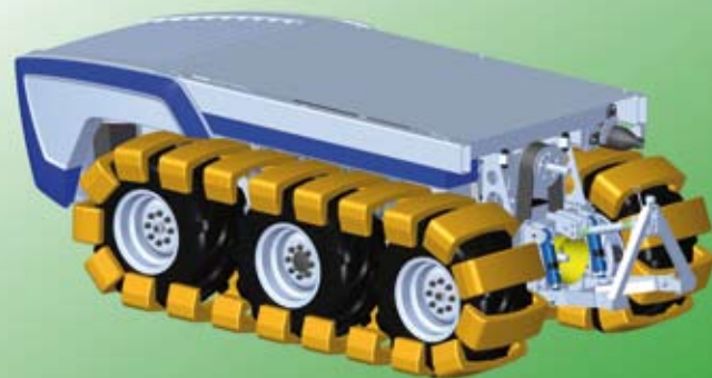
Fahrwerksvariante für schwere Bodenverhältnisse/ Equipment variant for pest management and soil management
